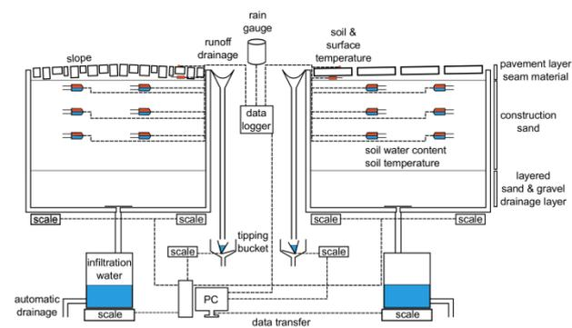
Figure 1: Lysimeter setup
