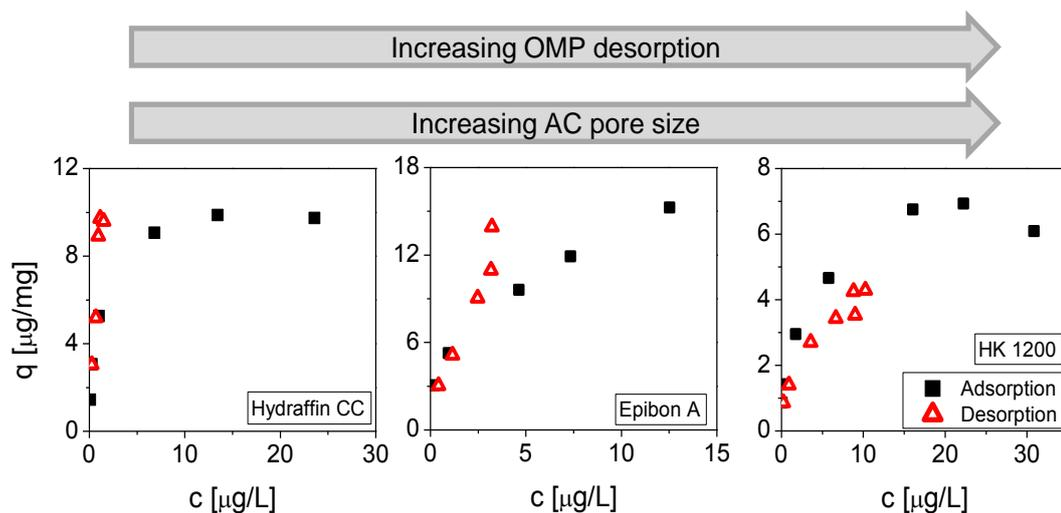
Figure 2: Adsorption and desorption isotherms of carbamazepine for three tested AC products (Hydraffin CC, Epibon A, HK 1200) from a batch experiment in Berlin drinking water; the shift of the desorption isotherm in comparison to its corresponding adsorption isotherm (from left/above to right/below) shows the increasing desorption from microporous Hydraffin CC to macroporous HK 1200.
