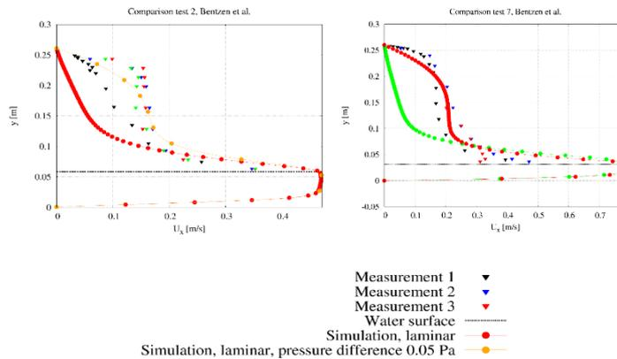
Figure 4: Comparison of simulated air phase velocities to experimental measurements
