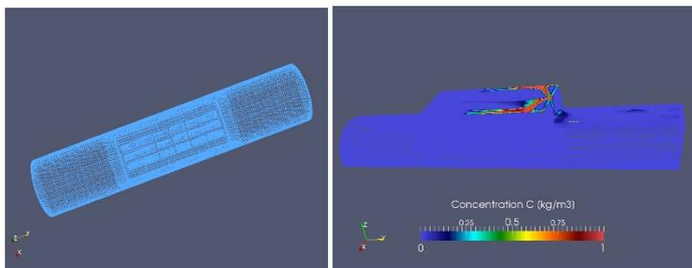
Figure 5: Transport simulations of flow around concrete probes (left: model domain with concrete probes; right: resulting tracer concentration)
