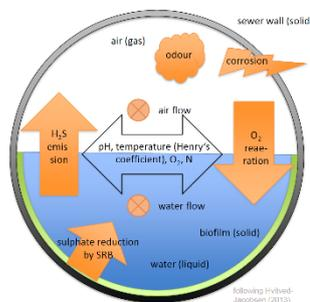
Figure 1: Overview over flow processes in sewer
