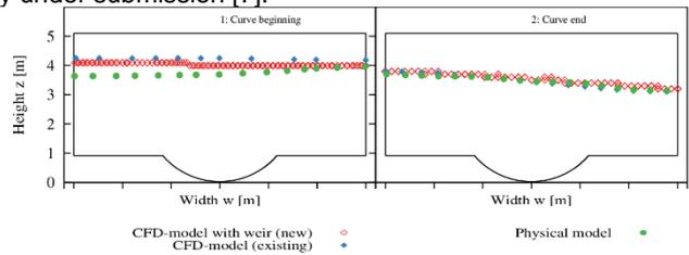
Figure 3: Comparison of water depths in complex sewer
