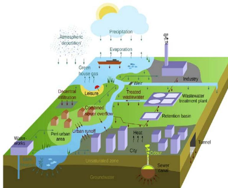
Fig. 1: Processes and elements within the urban water cycle [1, Gessner et al. 2014]
