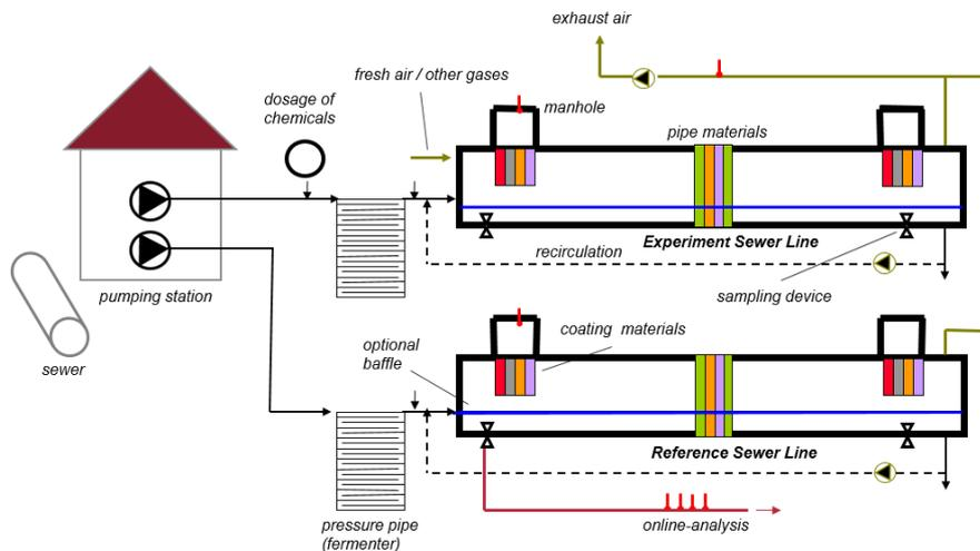
Figure 2: Schematic layout of the research sewer pilot plant (Barjenbruch et al. 2009)
