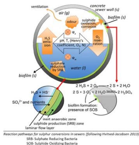
Figure 1: Overview of the formation process of hydrogen sulphide in sewer systems (UWI 2018)
