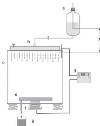
*Fig.1: Experimental setup for the rainfall simulation after Roder Green et al. (2014): (a) Mariott's bottle, (b) needle irrigator, (c) hermetically sealed plexiglas box, (d) data logger, (e) stainless steel tray, (f) digital scale, (g) runoff collection, and (h) pressure difference, adjusted*
