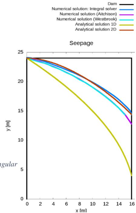
Figure 4: Dam geometry and seepages through a rectangular dam for numerical and analytical solutions
