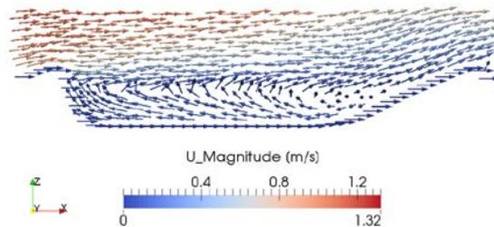
Figure 2: Velocity vectors for case 5 (ripple spacing)
