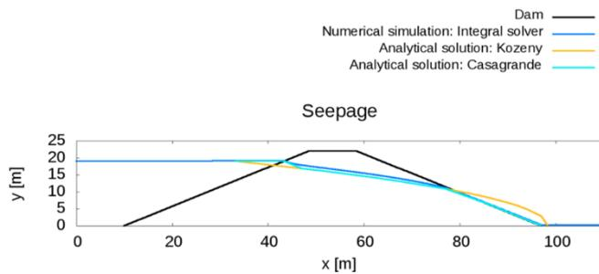
Figure 3: Dam geometry and seepages through a dam for the integral solver and two analytical solutions
