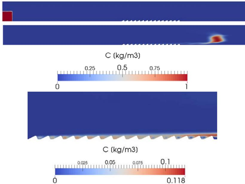
Figure 1: Tracer distribution at  $t = 0$  s (top) and,  $t = 10$  s from section  $x = 0$  m to  $x = 12$  m (center) and for the rippled area (section from  $x = 6$  m to  $x = 9$  m, bottom) for the reference case.
