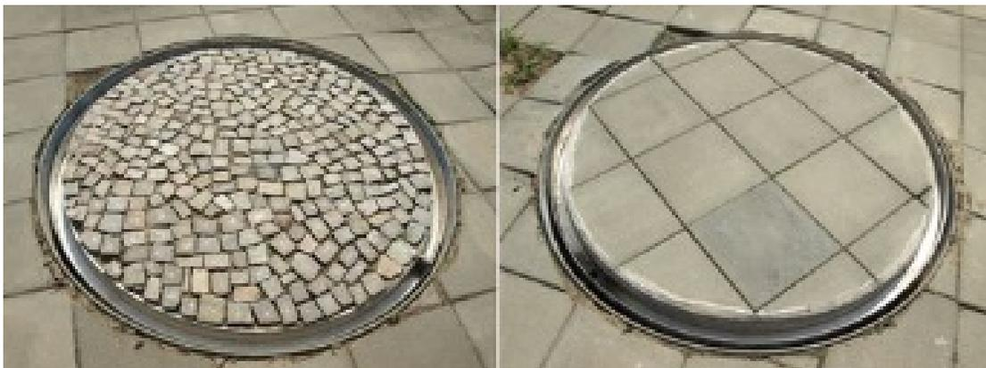
Figure 3: Two lysimeters with partially sealed urban surfaces studied in projects T1 and N2 (1st UWI cohort)
