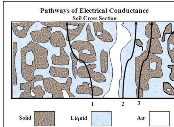
Figure 2: Three conductance pathways for the  $\sigma_b$  measurement. Modified from Rhoades et al. (1989)
