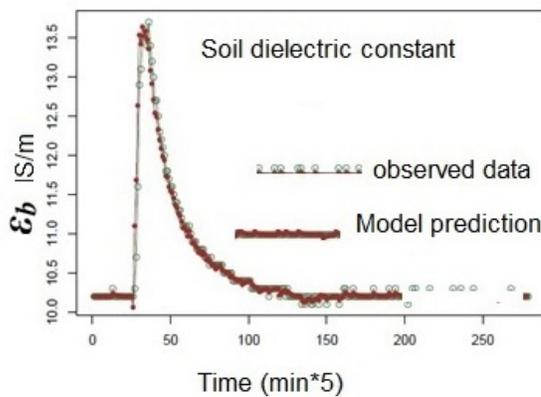
Figure 5: Observed and predicted soil dielectric constant at 21 cm depth.
